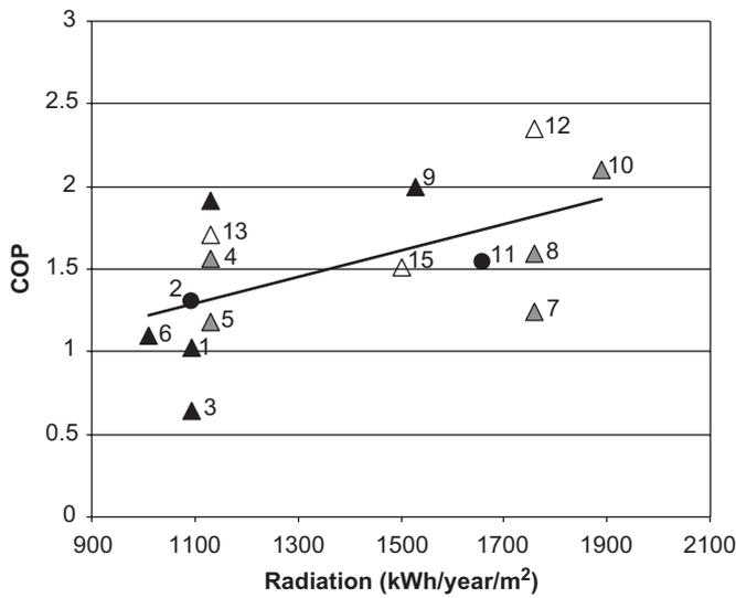
Fig. 2. COP versus solar insolation, solar systems.
