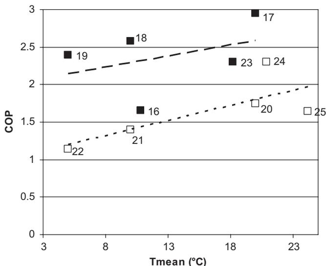
Fig. 4. COP versus ambient temperature, heat pump.
