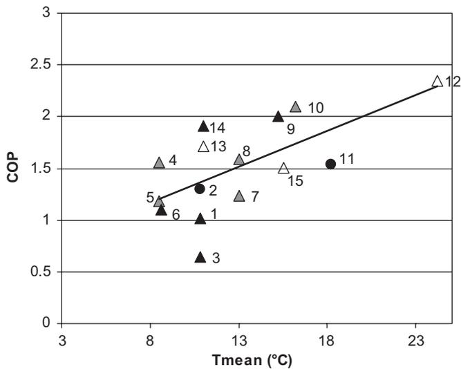
Fig. 3. COP versus ambient temperature, solar systems.
