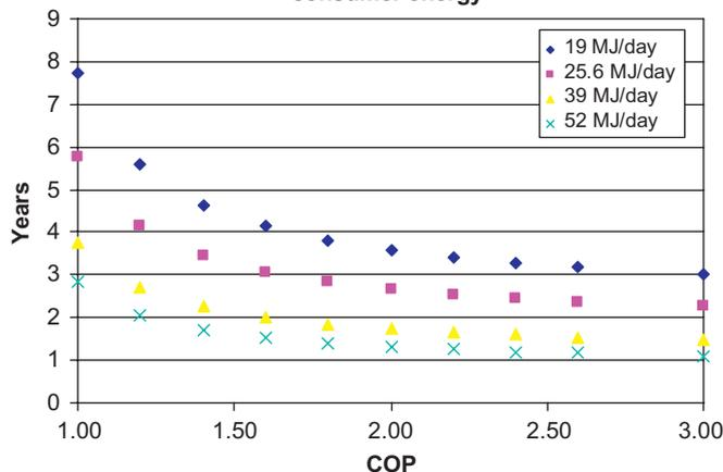
**Fig. 6.** Energy payback time versus COP and hot water usage for a flat plate solar hot water system using a conversion ratio of 1.5 between primary energy and consumer energy.
